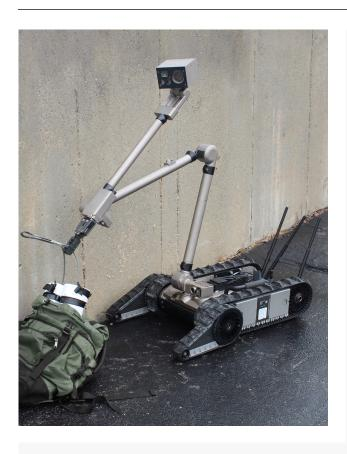
The PackBot 525 brings new and improved capabilities to the PackBot product line. Upgrades include state-of-the-art HD cameras, a laser range finder, optional in-situ charging, and more advanced accessory ports.
